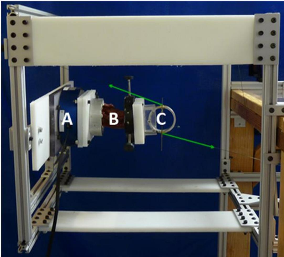
**Figure 1:** Biomechanical test jig to reproduce anatomical postures (neutral, flexion, extension). A) Load cell, B) Specimen, C) Pure moment fixture.
